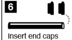
Insert end caps into both ends of the rail.
